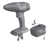
Push the battery into the tool from the rear until it engages with an audible click.
