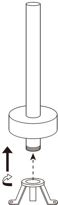
2. Screw the permanent seat onto the bottom
