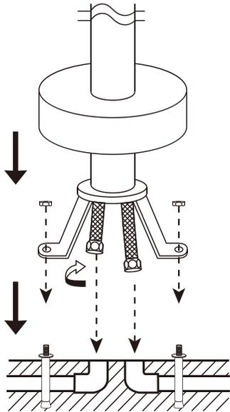
5. Tighten the screws to the permanent seat on the ground. Insert the flexible hoses into the hot and cold outlet tubes.
