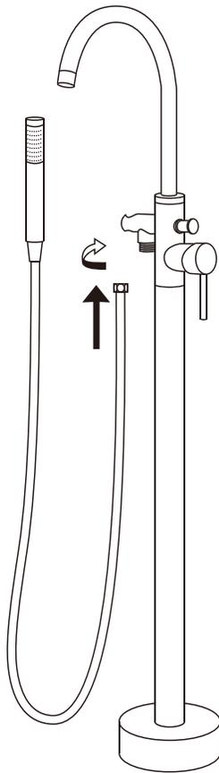
6. Install the hose to the hand shower and the tub filler. Please check that the tub filler spout, diverter and hand shower are functioning properly.
