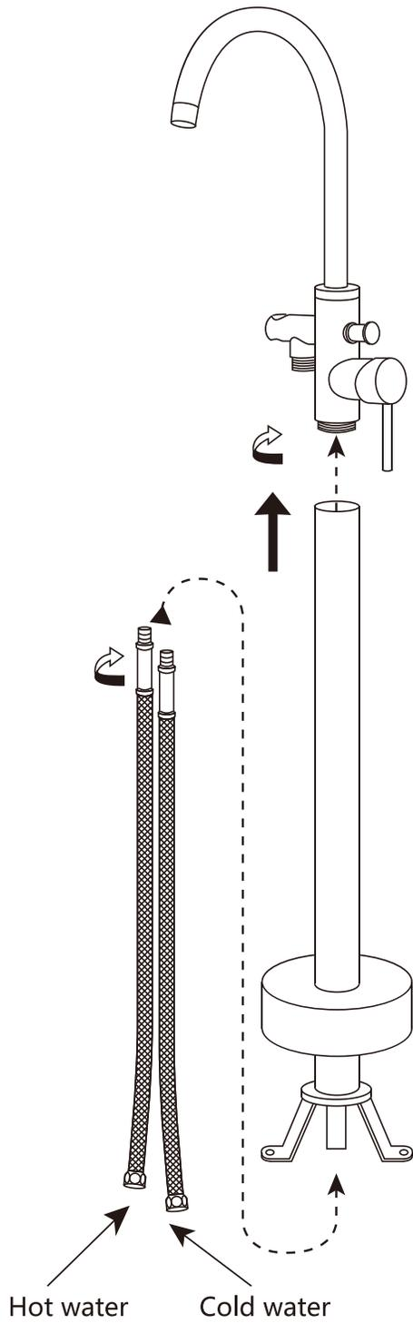
3. Pull the flexible hoses through the straight tube. Twist tight to attach them to the faucet.
