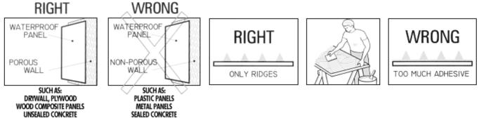
The water-borne family of adhesives, including latex and non-flammable based formulas, will not bond two impervious surfaces to each other, with the exception of Parkland Panel Adhesive. Because PLAS-TEX panels are impervious to moisture, the wall being covered must be porous enough to allow for adhesive drying. Wall finishes that are moisture proof must be removed or otherwise prepared to insure that there is adequate adhesive curing. Always follow adhesive manufacturer's directions completely.
