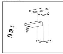
After installation is complete, remove aerator and rotate handle to the closed position. Turn on the water supply valves, and check all connections for a leak. Turn on your faucet and allow both hot and cold water to run at least one minute each. Replace Aerator.
