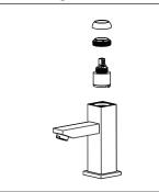
Remove handles. Unscrew Dome Cap counter clockwise by hand. Unscrew Retaining Nut using adjustable wrench, take out cartridge assembly and inspect. Replace parts as necessary. Reassemble parts by reversing steps.
