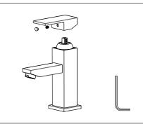
Turn off water and relieve pressure! Detach handle button using a small flathead screwdriver, unscrew set screw using Allen Wrench and take off handle.
