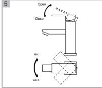
Lift the handle up, the cartridge will be activated allowing water to flow. The water flow will increase by continuing to rotate handle. By rotating the handle to the right, the water temperature will decrease to cold flow only. By rotating Handle to the left, the water temperature will increase to hot only.
