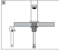
If necessary, tighten screws using a adjustable wrench until the faucet is firmly connected to the sink.
