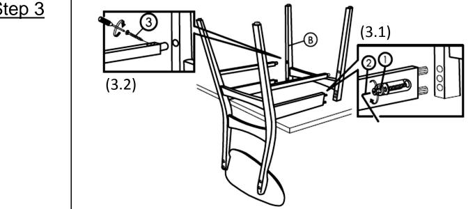
Place the Front Leg (B) on the Side Stretcher and Side Rail as shown.
