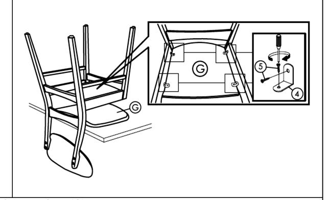
Place the Cushion Seat (G) on the table and put the chair on it as shown. Then, fix the Cushion Seat (G) with L-Bracket ④ and Screw ③ using Screwdriver (not provided).
