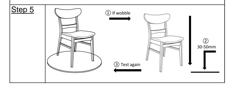
Place the dining chair on a Level Surface to check if it wobbles. loosen the bolts and lift the dining chair some 30cm to 50cm high from the ground, keep your feet and toes well away from the drop zone, and drop the dining chair freely and vertically with the four legs, hitting the ground at the same time.
