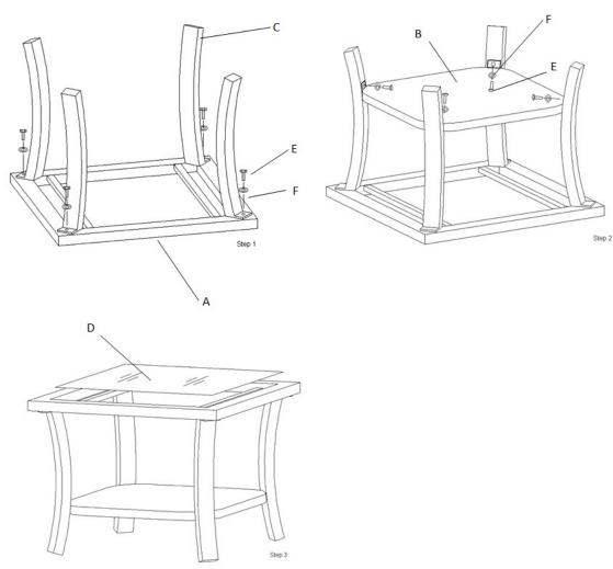
Important: please do not tighten any screws until all the screws are in the right position.
