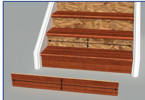
8. As in step #6, use heavy duty all urethane construction adhesive. Apply about an 1/4" thick bead around the perimeter and then throughout the middle in a zig-zag shape on the back of the riser as previously shown and adhere the riser to the existing riser.
