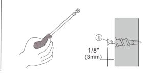
**Stud Mounting**(1b)Using a stud finder, locate and carefully mark the location of studs on the wall where you want to hang your shelf.
