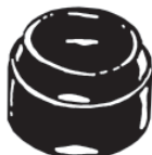
Upper Shaft Seal O.D. - 1" I.D. - 3/4" Thickness - 1/2"
