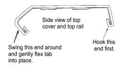
\*Bullnose rail is used for the illustration, but installation is the same for all 1 pc. clip-on resin covers.
