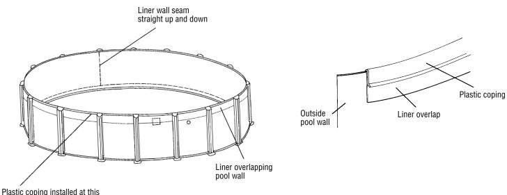
Plastic coping installed at thi time to hold liner in place
