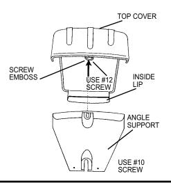
1) Attach the inner top cap using a #12 Screw into hole #2. See diagram below
