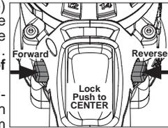
To **lock** the trigger, push the control switch to the center position. The trigger will not work while the control switch is in the center locked position. Always lock the trigger or remove the battery pack before performing maintenance, changing accessories, storing the tool and any time the tool is not in use.
