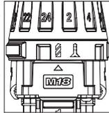
2. To use the **driving screws mode** rotate the application selector collar until the drive symbol
