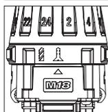
The adjustable clutch, when properly adjusted, will slip at a preset torque to prevent driving the screw too deep into different materials and to prevent damage to the screw or tool.
