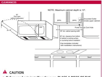
Before you begin installing the oven, PLACE A PIECE OF THE CARTON OR OTHER HEAVY MATERIAL (a blanket) over the countertop or cooktop to protect it. Do not use a plastic cover. Failure to protect these surfaces could result in property damage.
