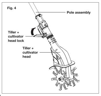
⚠WARNING! Make sure nuts, screws and locks are properly tightened before using the cordless tiller + cultivator.
