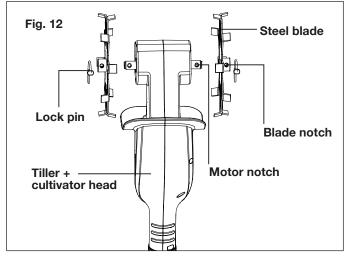
3. Insert the new blade onto the motor shaft. Make sure to align the notches on the blade's hole with the notches on the motor shaft (Fig. 12). Then, slide the lock pin into the holes of the blade and motor shaft to keep the blade in place. Close the ring over shaft to lock the pin. Insert the battery and resume working (Fig. 13).
