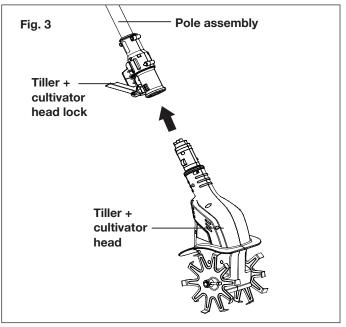
2. Flip up the tiller + cultivator head lock to lock the tiller + cultivator head in place (Fig. 4).
