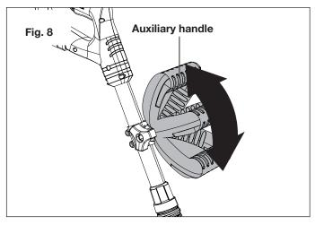
Turn the handle knob back to lock the auxiliary handle in position.
