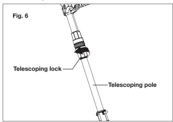
2. Lock the telescoping pole in position by turning the telescoping lock counterclockwise, and ensure that the pole is secured.
