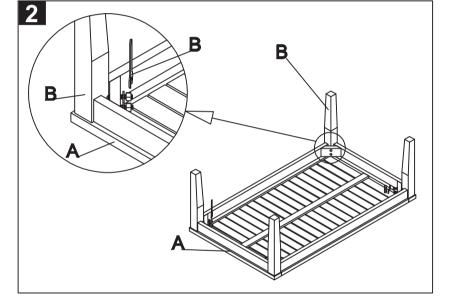
Step 1: turn the table top and put the 4 legs (B) on the table top (A).
