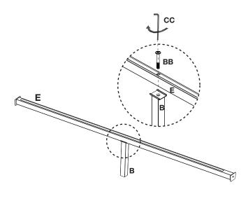
$\hfill\Box$  Insert connecting pipe (E) into slots of horizontal tube (C) as shown.
