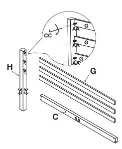
□ Joint headboard horizontal tube (G), horizontal tube (C) to another headboard leg (H) with bolt (AA).
