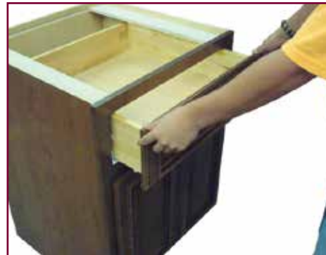
3. Insert drawer and fully close. Open and close repeatedly to align runners.
