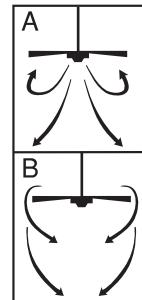
NOTE: Turn off and wait for fan to stop before changing the setting of the forward/reverse slide switch
