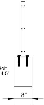
Use epoxy anchors instead of wedge anchors for gate shoe
