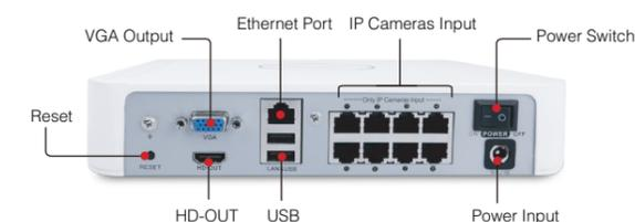
**VGA Output** : Connect to your TV or computer monitor via VGA port.
