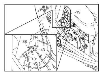
Slightly loosen the indicated M4 x 16mm Screw (101). Slide the Reed Switch (38) slightly closer to or away from the Magnet (43), and then retighten the Screw. Then, plug in the power cord, press the power switch to the reset position, and rock the Pulley (19) forward and backward just enough that the Magnet passes the Reed Switch repeatedly.
