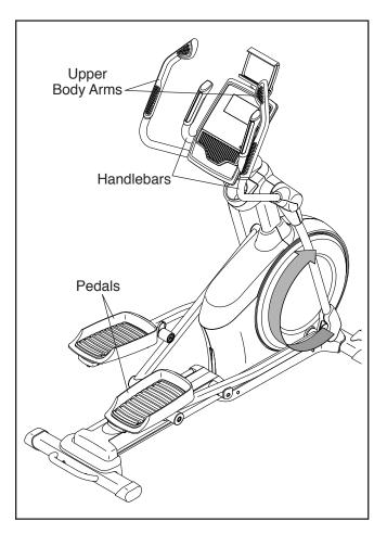
To dismount the elliptical, wait until the pedals come to a complete stop. **Note: The elliptical does not have a free wheel; the pedals will continue to move until the flywheel stops.** When the pedals are stationary, step off the higher pedal first. Then, step off the lower pedal.
