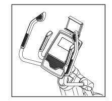
holder to the desired angle. Reverse these actions to remove the tablet from the tablet holder.
