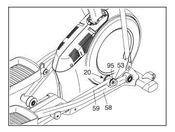
**See EXPLODED DRAWING C on page 35.** Identify the Left and Right Shields (73, 74). Remove the M4 x 19mm Screws (5), the M4 x 25mm Screws (127), and the M4 x 48mm Screw (107) from the Left and Right Shields; **make sure to note the location of each size of Screw.** Then, remove the Right Shield.
