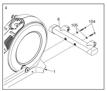
Tip: Avoid pinching the Main Wire (110). Avoid damaging the indicated plastic tabs (A). Have a second person hold the Upright (4) on the Frame (1).
