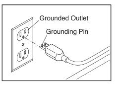
The outlet must be on a nominal 120-volt circuit.
