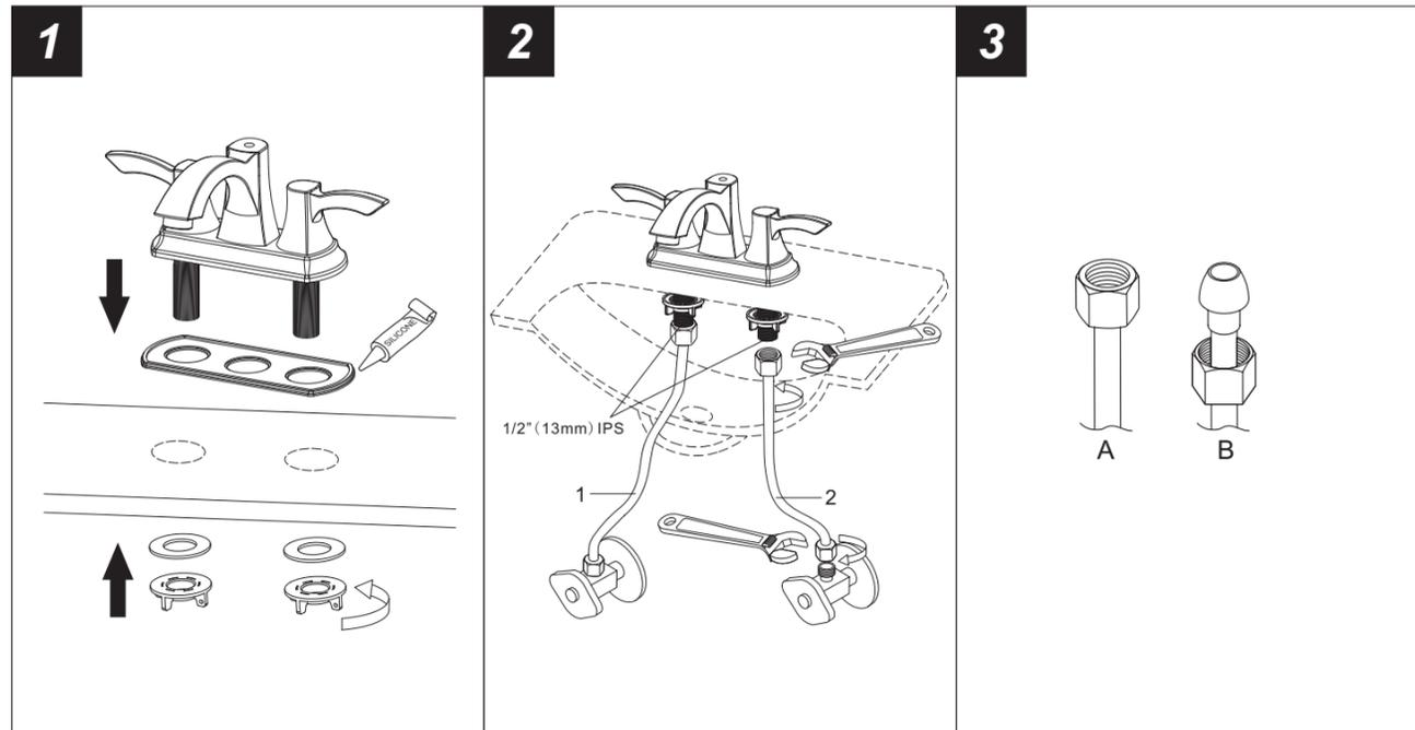
1. Place the faucet and gasket on the basin, from underside of basin, assemble the washer and lock nut, tighten the lock nut by hand. **If the basin is uneven, please use silicone under the gasket.**
