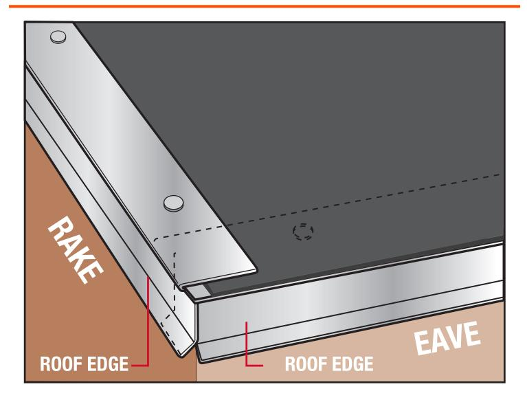
Begin installation along the eaves, starting at a corner and working your way around, overlapping each succeeding piece of drip edge by 2-3 inches.
