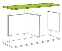
Start with the bottom horizontal zBoard (there will be holes on only one side of board).
