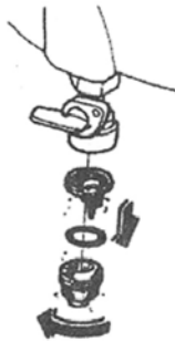
Fuel Filter Element Removal
