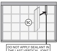
D. Apply a 1/4" bead of sealant horizontally across the top of the opening 1/2" from the face of the glass blocks. This sealant line will be used to secure the second half of the top channel.
