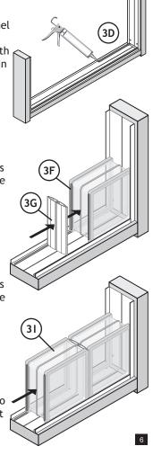
J. Continue inserting spacers and blocks in this manner to complete the row. Do not apply sealant to the side of the last block and last spacer. Insert the last block in the side channel and slide it into the bottom channel.
