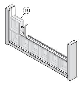
C. Install the remaining rows in this manner until you reach the last row. Check each row for alignment vertically and horizontally.
