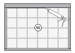
E. Apply a 1/4" bead of sealant along the top inside leg of the second half channel.
