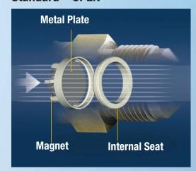
In standard operating conditions, the magnet holds the metal plate in place, allowing gas to flow to the appliance.
