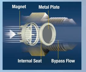
A gas line rupture produces an unrestricted gas flow through the valve, forcing the plate away from the magnet. The plate seals firmly against the seat, immediately restricting gas flow to avert a hazardous release of gas into the home.
