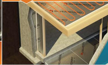
SilveRboard UC has an R5 per inch and compressive strength of 35 PSI making it the ideal solution for under concrete slab application. SB UC is laminated on the down side with a reflective film and on the concrete placement side with an opaque grey film, this film provides added strength, a vapour barrier and radon barrier (when taped as per specification) and reduces job site breakage and cracking during the construction process.
