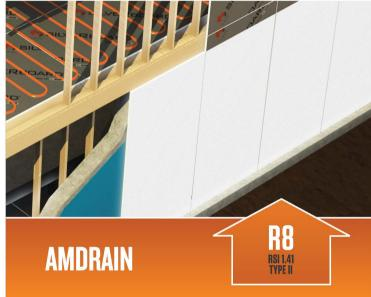
Amvic AmDrain foundation insulation board is an EPS (expanded polystyrene) panel with one flat side and one side vertically grooved to provide a drainage system for either exterior or interior insulation, it is used as a supplementary component in all types of foundation / basement building systems.
