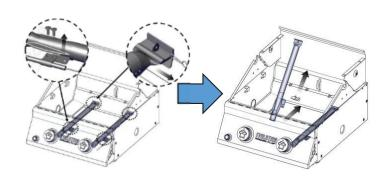
**Step 2.** Reinsert the new burner onto the orifice, as shown below, make sure burner hole aim at orifice. Repeat the procedure for the each burner.
