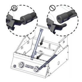
**Step 3.** Reattach gas burner using screws and cotter pin.
