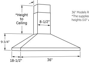
36" Models Require a 36"-Wide Opening \*The supplied duct cover fits 7'-4" to 8'-10" ceiling heights (10" with optional high ceiling kit JXDC72)
