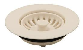
Remove any old strainers or screens from sink. Insert the RP32125WH strainer in the drain hole in sink. Push down firmly to seal the strainer to the sink. To allow for faster drainage, turn center knob and lift up, pulling the center straining basket out.
