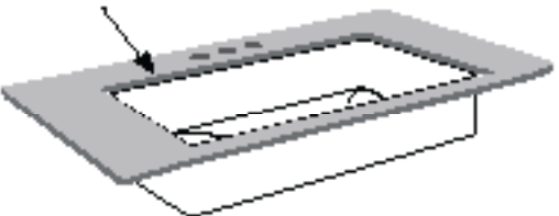
VERIFY SINK IS CENTERED WITHIN THE COUNTERTOP OPENING BEFORE TIGHTENING FASTENERS.
