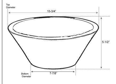
Dimensions of fixture are nominal and may vary within the range of tolerances established by ASME Standard A112.19.2. Dimensions and specifications subject to change without notice.
