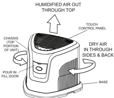
Dry air is drawn into the unit through the sides where the air is pulled through the saturated wicks and becomes moisturized before it is fan forced out the top of the unit into the room.
