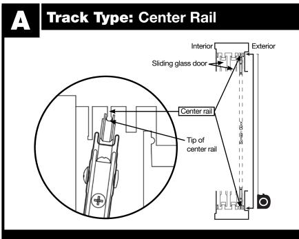
Measure tip to tip of center rail at top and bottom of sliding screen door track
