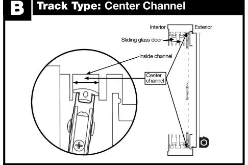
Measure inside cemter channel to inside center channel at top and bottom of sliding screen door track
