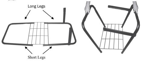
5. Attach the other end of the LEG BRACES to the corresponding legs using 1 3/4" Hex Bolts and Nuts but only finger tight. See below.
