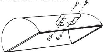
12. Set the HOOD, in the CLOSED POSITION, on top of the bottom Half of the grill body. Line up the Hinge holes and insert the Hinge Pins. This may require lifting up on the back of the Hood. Then, carefully open the hood, making sure to not let the Hinge Pins fall out, and insert the Hair Cotter Pins into the Hinge Pins. See below.
