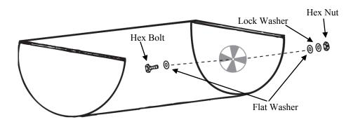
14. Attach SIDE SHELF to the four (4) holes on left side of grill with 1/2" hex bolts and nuts. See below.
