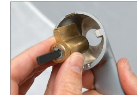
4. Slide the handle onto the drive shaft until it hits the catch pins.
