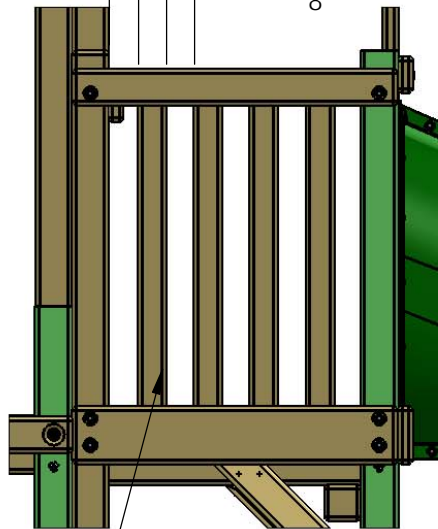
5/4 X 3 X 34-1/2" PANEL SLAT (4 ON RIGHT SIDE)
