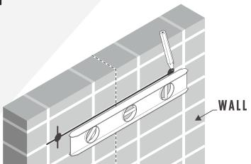
Once position is marked, drill 2 holes and insert anchors if stud is not available
