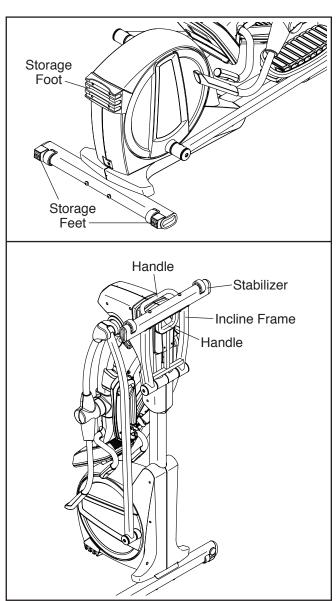
To lower the elliptical for use, first hold the handle on the incline frame with one hand and hold the front stabilizer with your other hand. Next, pull the frame towards you and lower it until you can reach the handle on the front stabilizer. Then, hold the handle on the front stabilizer with both hands and finish lowering the elliptical to the floor.
