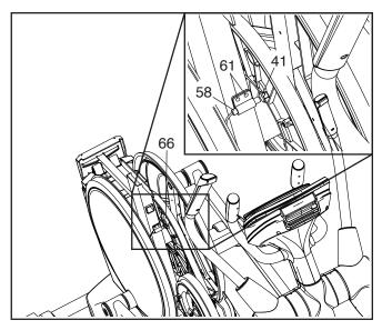
Slightly loosen the two indicated M4 x 16mm Screws (61), slide the Reed Switch (58) slightly toward or away from the Magnet (41), and then retighten the Screws.
