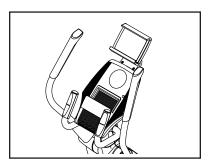
**tablet holder.** Rotate the tablet holder to the desired angle. Reverse these actions to remove the tablet from the tablet holder.
