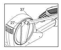
Screws (not shown) from the Top Shield (37), and then use a standard screwdriver to pry the Top Shield upward off the elliptical.
