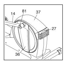
Next, remove the four M4 x 16mm Screws (not shown) from the Large Storage Foot (27), and then remove the Large Storage Foot. Remove the two M4 x 16mm Screws (not shown) from the Top Shield (37), and use a standard screwdriver to pry the Top Shield upward off the elliptical. Then, pry the left Pedal Disc (36) off the elliptical.
