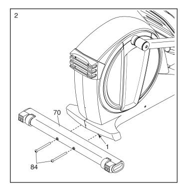
3. With the help of another person, place some sturdy packing materials under the front of the Frame (1). Have the other person hold the elliptical to prevent it from tipping.
