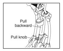
Next, pull the upright forward slightly, lift the latch, and then lower the upright to the folded position. Hold the upright in one of the indicated locations while you lower the upright; do not hold the upper body arms.
