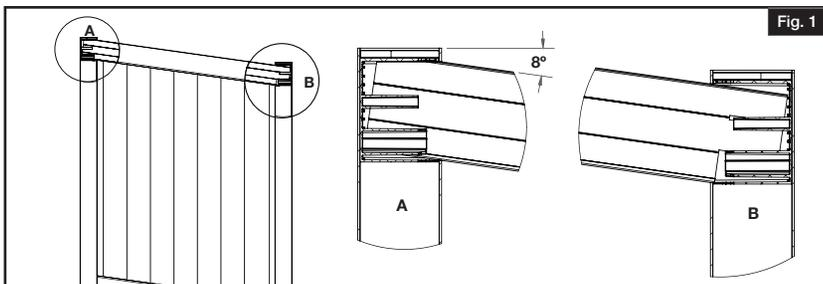
**4** Screw the assembly together, and let compound cure until dry.
