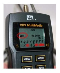
**SPLIT PAIR**: Indicated by having the pairs that are split flash on and off on the LCD with the Split icon lit.
