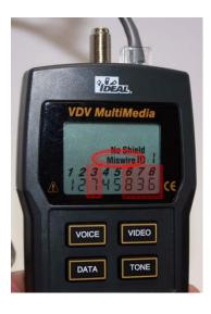
MISWIRE: or reverse. Indicated by a two or more different pin numbers below the top number. What it means: Conductors are in wrong order.
