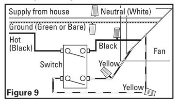
**NOTE:** The fan's receptacle wires might need to be pulled outside compartment for connection. Only pull the five loose wires outside of compartment. Additional wires will be present.
