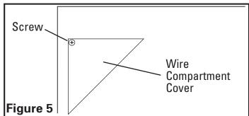
1b. Internal Wire Compartment: Using a 7/16" socket, remove the two hex nuts holding the blower assembly in place. Lift up on the assembly and slide it out of the tabs on the housing (Figure 6). Remove the wire compartment cover screw and place the cover in a secure place (Figure 7).
