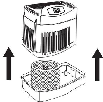
3. Grasp the housing assembly and lift straight up and away from the base and set aside. The wicking filter is now accessible.
