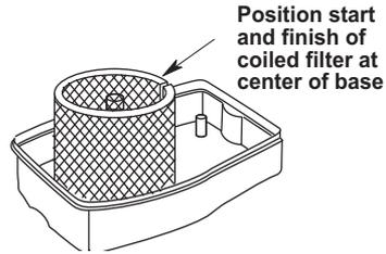
5. Install a new wicking filter (MAF2) into the base. Coil the filter and position it between the uprights in the bottom of the base. The start and finish of the coil should be captured at the center of the base (see diagram) and the filter should be resting on the floor of the base.
