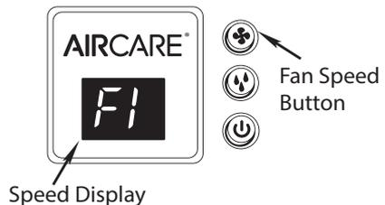
The selected setting is displayed on the digital readout. The higher the setting, the faster water is evaporated and released into the air. **F1 (LOW)** is the quietest setting and is provided for conditions that do not require a rapid evaporation rate.
