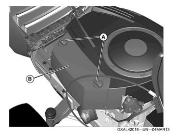
5. Lift latch (A) to unlock cover (B). Lift cover forward and remove.
