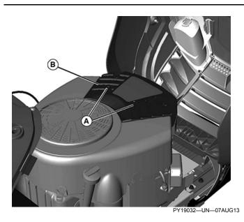
5. Loosen knobs (A) and remove cover (B).
