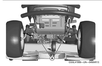
Secure front of machine at both sides of the axle at points (A) to trailer with heavy-duty straps, chains, or cables. Straps must be directed down and outward from machine.
