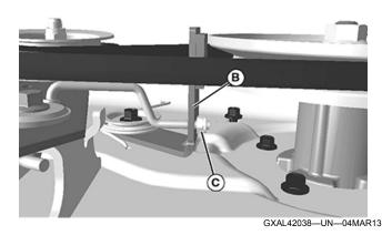
Measure distance from spindle brake bracket (B) to nut (C) on end of brake rod.
