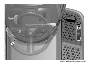
Push and hold in the reverse implement switch (A) while depressing reverse pedal slightly for hydrostatic transmission or moving the transmission shift lever to the rear slot (reverse) for automatic transmission.
