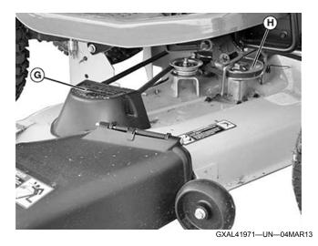
3. Top of mower deck, under shields (G), including spindle (H) and belt areas
