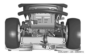
Safely lift and support machine. Place safe lifting device under end of front hanger bracket at location (A), and place jack stands or other stable supports under frame on each side at location (B). Block wheels remaining on the ground to prevent machine movement.
