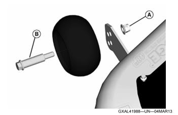
Check each mower wheel position. Remove nut (A) and bolt (B), and move mower wheel to proper hole.
