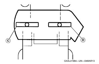
Turn left blade (C) as shown. Hold drive belt and turn right blade (D) as shown. Take measurement for both blades.
