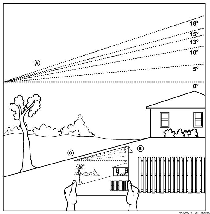
Use this slope gauge to determine if a slope is too steep for safe operation. Do not operate your machine on a slope greater than what is recommended in your Operator's Manual. See Operating on Slopes in the Safety Section.
