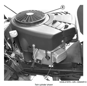
2. Engine intake screens (E), cooling fins (F), and oil cooler (if equipped).
