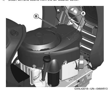
5. Loosen two knobs (A) and remove cover (B).
