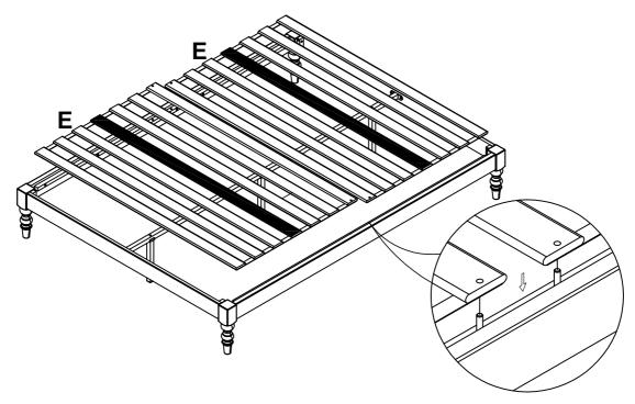
8.Remove adhesive covering from the 2 pieces of slate. The assembly of the bed platform is complete.
