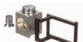
Neutral Lug Kit, ECLK1-2 wire range — #2-1 AWG Cu or Al
