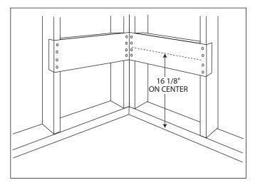
NOTE: After installing the 2 x 6 wall support, finish out the wall with drywall and a Swanstone wall panel system or a wall covering of your choice. After the wall covering has been installed, set, and allowed to cure, move on to Step 3.
