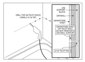
5. Use the 3/8" drill bit to enlarge the 3/16" pilot holes through the Swanstone wall panel or other wall material. Only drill the 3/8" holes through the thickness of the wall panel. Do not drill into the 2 x 6 inch wall support.
