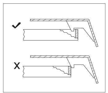
b. If the wall corner is not exactly 90 degrees square, it will be necessary to sand the sides of the seat in order to achieve a proper fit. Use a coarse grit (60 grit) sandpaper when sanding the seat.
