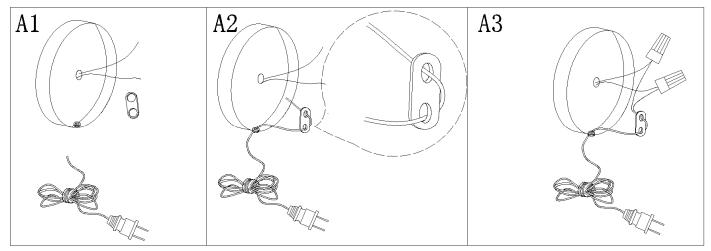
Step A1: Pass the power cord through the hole in back plate
