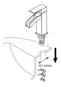
2 According the remove step to screw up the fixing set to the mixer below the basin.
