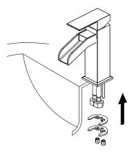
**3** Use hand to screw up the locknut, then use install tool for fixing strengthen.
