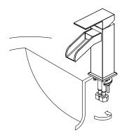
4 Connect the inlet hose from the body, "Red" for connecting to the hot water, and "Blue" for connecting to the cold water.
