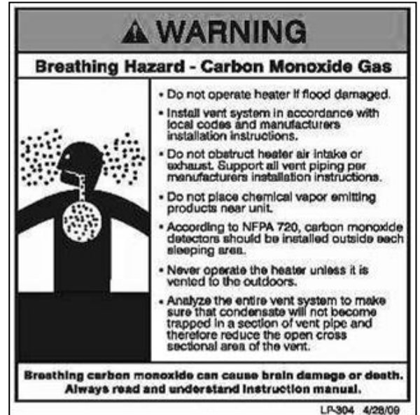
Figure 3 – CO Warning Label
